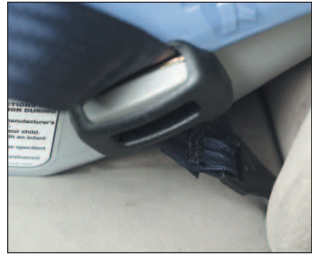
Flexible LATCH hook using anchor bar
